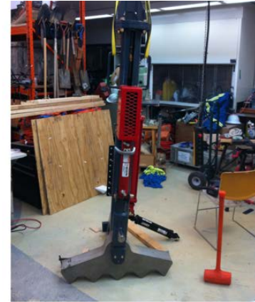
FIG. 2. The USAInC compressed nitrogen accelerated weight-drop source as delivered. Lawton et al., 2013
