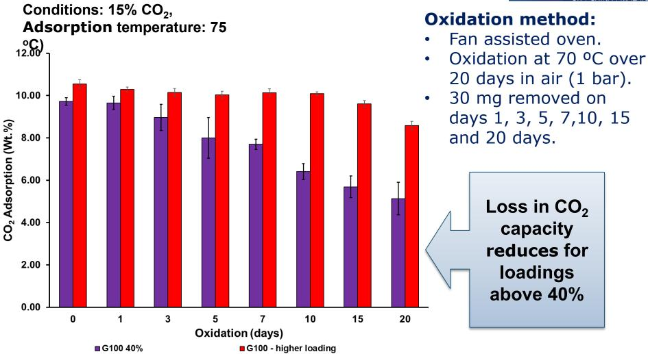
• 47% drop in CO<sub>2</sub> capacity after 20 days oxidation with G100 40% loading.
