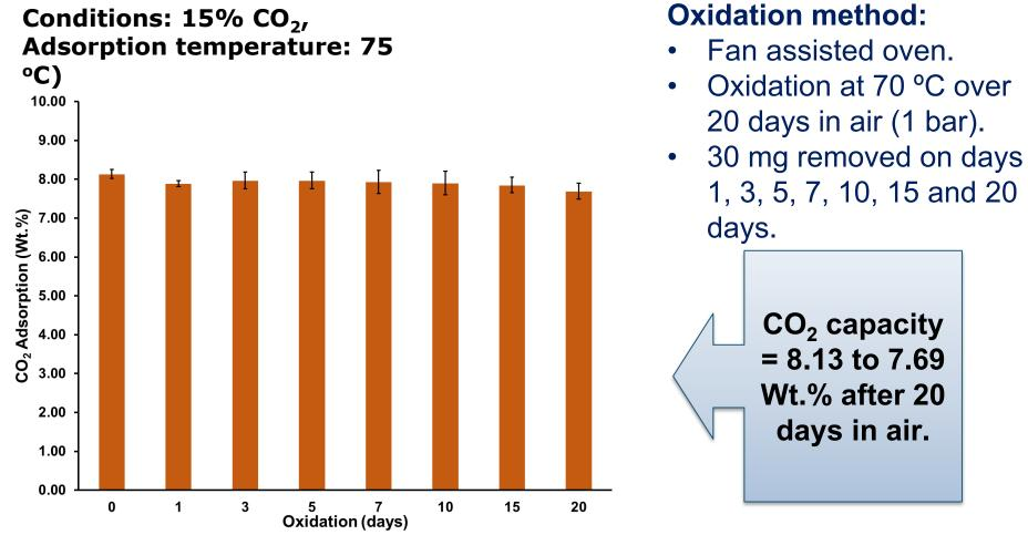
• Only 5.4% drop in CO<sub>2</sub> capacity after 20 days oxidation.
