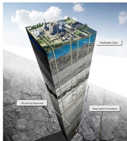
Figure 1: Geological storage of CO 2
