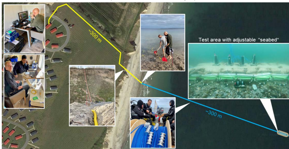
Figure 2 Design, installation, data acquisition and interpretation of seabed displacement with Distributed Strain Sensing fibre optic cables in offshore Germany.
