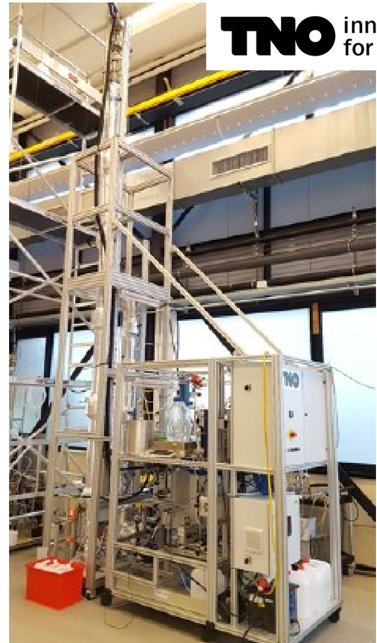
Larger test rig for operating TNO's STAR solvent
