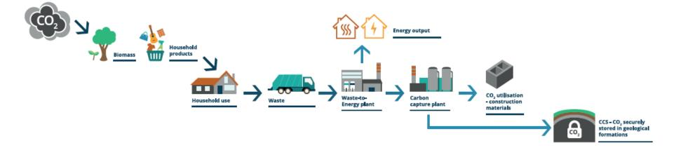
How CO<sub>2</sub> from biogenic sources of waste can create negative emissions if it is captured and stored securely
