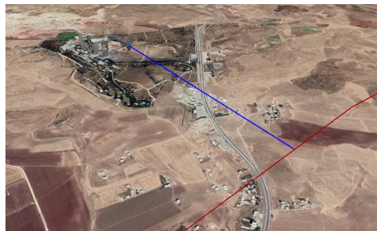
Limak Cement Factory to Dodan CO 2 Pipeline, 1.8 km Estimated emission: 400,000 tonne CO 2 /year
