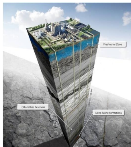
Figure 1: Geological storage of CO 2
