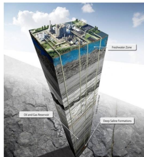
Figure 1: Geological storage of CO 2
