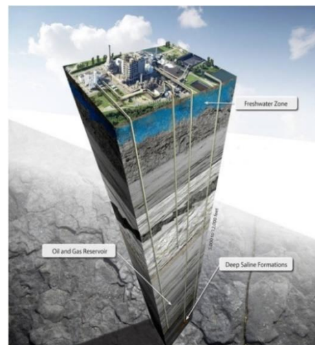
Figure 1: Geological storage of CO 2
