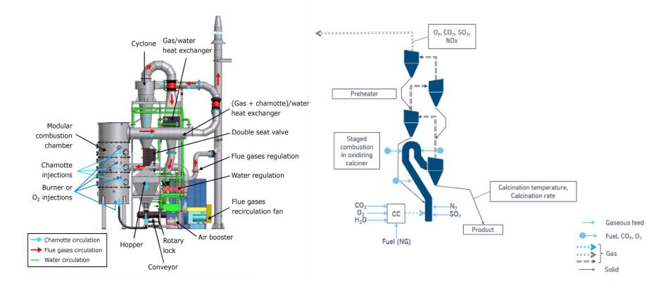
Schemes of pilot scale oxyfuel calciner facility from Air Liquide & TKIS
